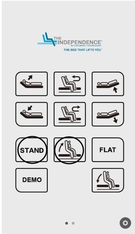
Tap and hold the
